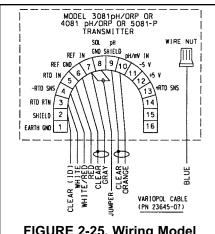
FIGURE 2-25. Wiring Model 396VP and 398VP to Model 3081 and 4081
